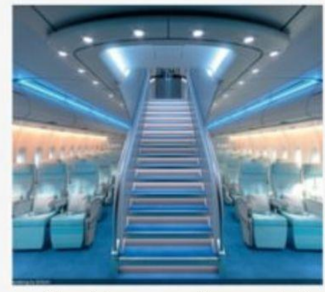
Two staircases provide access to the aircraft's upper and lower decks
